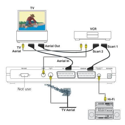
You can now record digital terrestrial television programmes by selecting SCART 1 on the VCR. The VCR will also be able to record analogue television channels in the usual way. Both live and recorded digital terrestrial television programmes can be viewed on the TV by selecting the TV's AV input.
